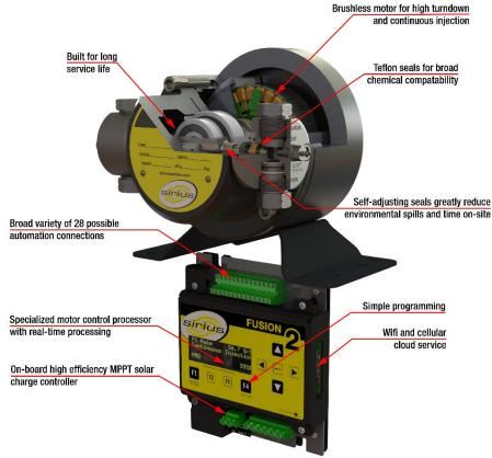
Figure 2: Smart pump, motor, and controller
