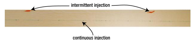
Improved dispersion through continuous injection best assures that the closest to ideal injection rate can be used to fully treat the flow stream. In real world applications, operators have reported significant performance gains after retrofitting from an intermittent to a continuous pump:
