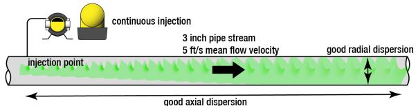
This uniform and continuous flow maximizes the chemical contact time with the flow stream, and. ensures the chemical has the best opportunity to disperse both radially and axially in the flow stream. Most chemical treatments become more effective as contact time increases. By ensuring
