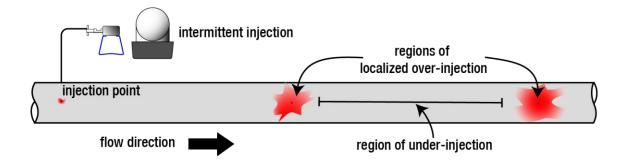
Most chemical pumps today are controlled by a timer to achieve a given number chemical doses per minute. For example, a pump that outputs a maximum of 100 Q/d would run 10% of the time to output a desired value of 10 Q/d. The on/off timer would run the pump on for, say 1 second, and off for the next 9 seconds of a 10 second cycle.
