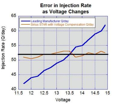
fluctuates. Adjustments can be made to either the "ON" time of the chemical pump, or to the average RPM of the motor in order to consistently deliver a calibrated rate.
